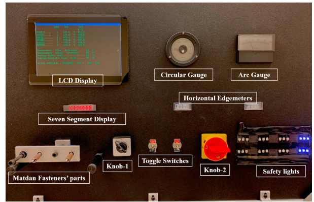
Fig. 3: Mock panel built with various factory floor artifacts
